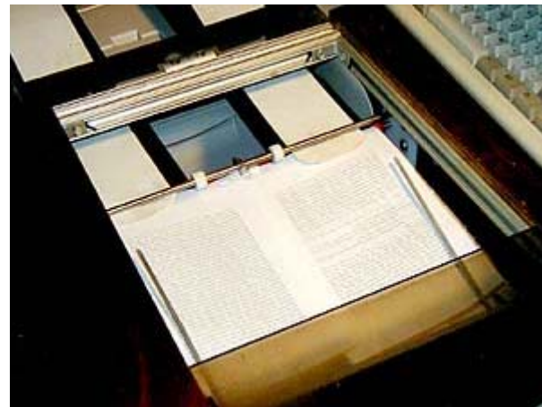
A page being split. This page is being conveyed from the printer (outside of the photo at the top) to the collection tray. On the way, it passes under a splitting wheel (centered between two white plastic pressure wheels) which divides the 8.5'11-inch sheet into two 5.5'8.5-inch book pages.
