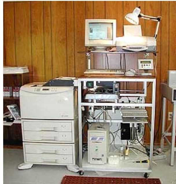
Inside the InstaBook Maker. Pages are produced on the printer at left. They are split as they pass from the printer to the collection and gluing station in the center (above the PC that controls the system). The cover jig, where the operator places the cover prior to binding, is at the right side of the machine. The ink-jet printer on which covers are printed is at the top, under the lamp.
